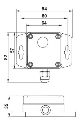
The IP65 instrument sensor is equipped with a hydrophobic microporous PTFE filter to protect the sensor from dust, dirt, and water drops.
